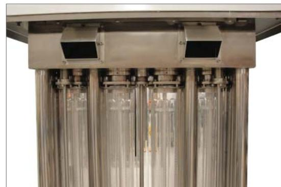
The MicroDynamics® automatic wiper system is chemical-free and uses a motor driven stainless steel assembly.
