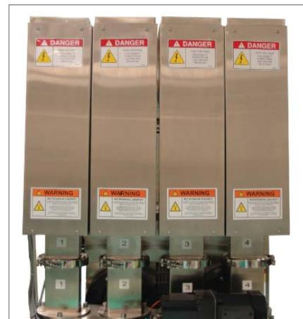
Integrated heads contain the power supply and magnetron.
