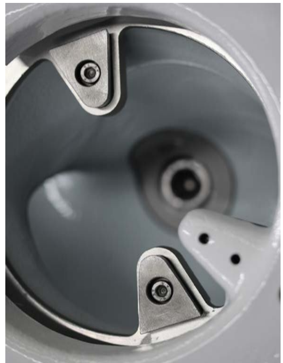
The ASC system has replaceable hard metal blades (HRC 55).
